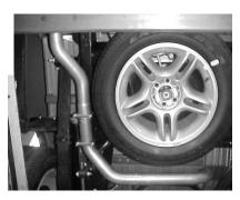
INSTALL DRIVERSIDE FRONT TAILPIPE #B INTO MUFFLER AT LEAST 1 1/2" TO 2".USING CLAMP # F. NEXT INSTALL DRIVERSIDE OVERAXLE PIPE # C TO FRONT TAILPIPE USING CLAMP # F DO NOT TIGHTEN
